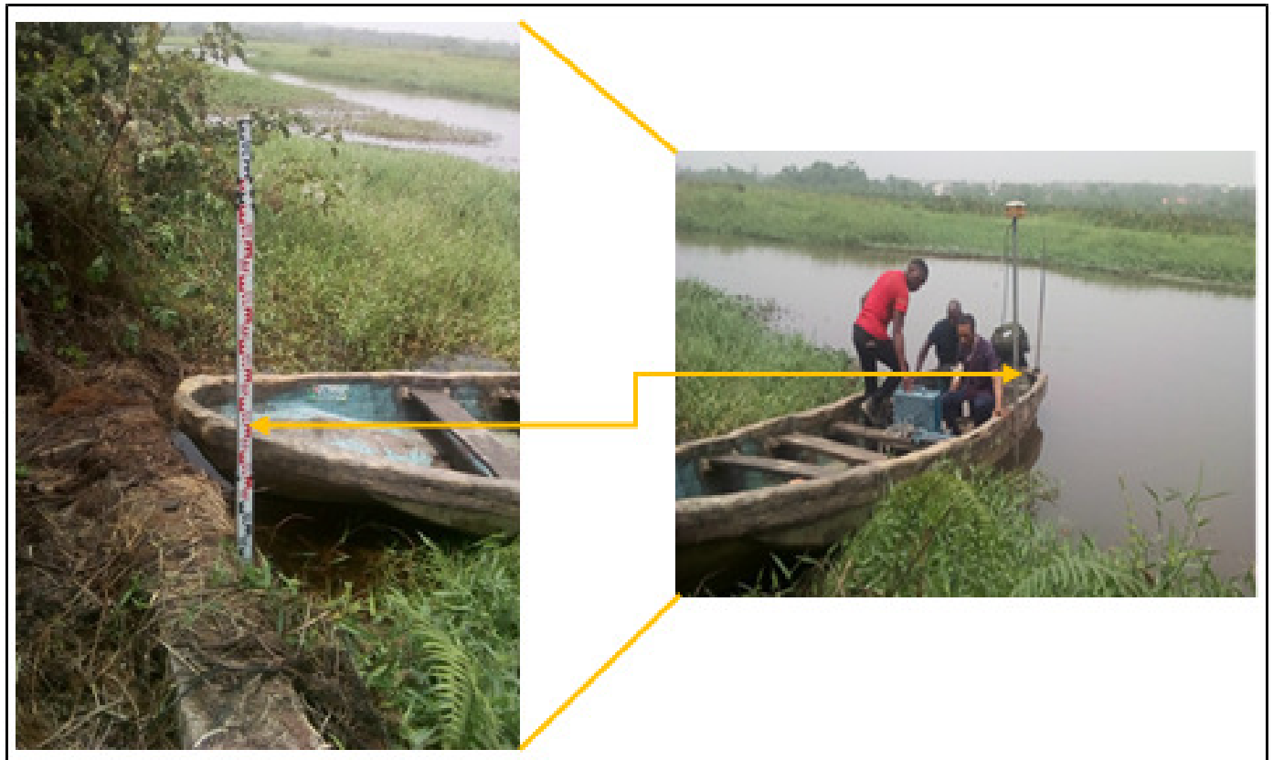
Figure 5. Bathymetric survey and water level monitoring exercise at Ikpoba dam
