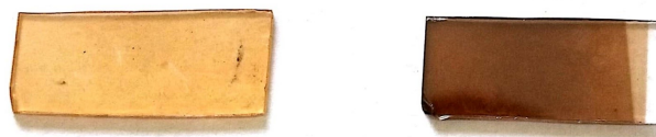
Figure 1: Surfaces of the undoped (left) and Cu-doped (right) \text{Fe}_2\text{O}_3 deposited films taken by an optical camera Camon 12 Pro.
