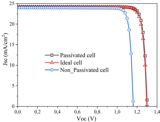
Figure 4: I-V characteristic of the simulated module
