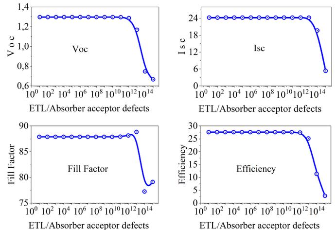
Figure 2: Effects of acceptor defects density at ETL/Absorber interface
