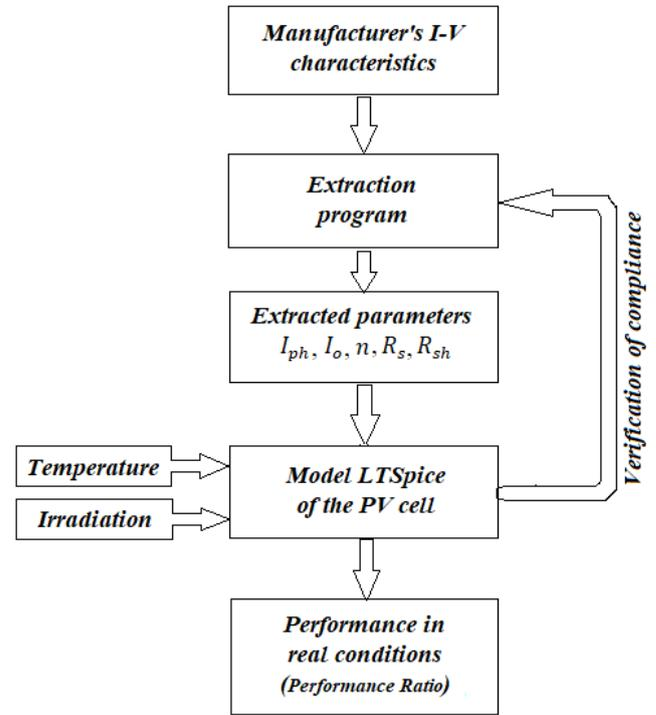
Figure 1: Diagram of the performance ratio evaluation
