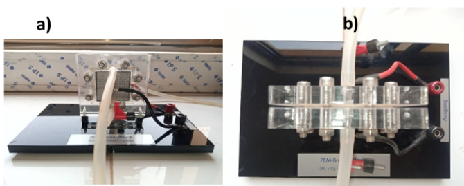
Figure 3: Fuel cell : (a) view from the side and (b) View from the top
