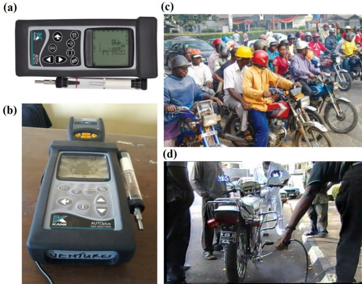
Figure 2. (a-b) KANE Automotive 4-Gas Analyzer (Model 4-2) used; Photographs of (c) typical motorcycle taxis terminus (d) field exhaust emission test of the sampled motorcycles.
