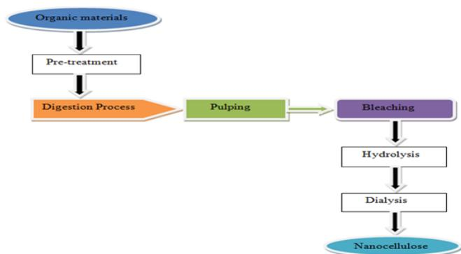
Figure 1. Schematic Diagram of Experimental Procedure of nanocellulose
