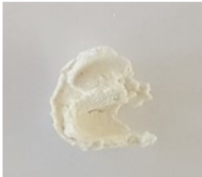
Figure 4: Prepared Zinc metal soap sample.
