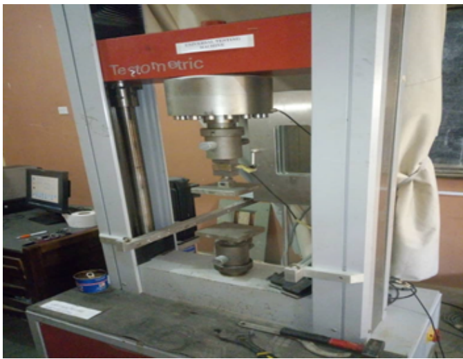
Figure 2. Testometric Compression Test Machine used
