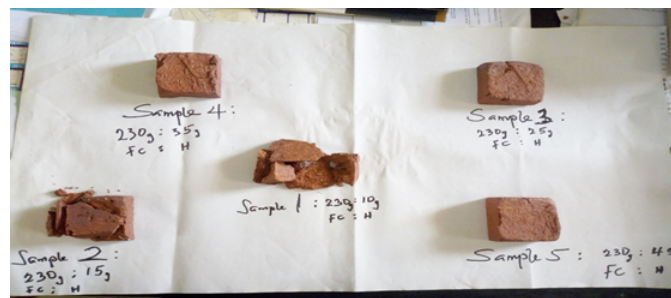
Figure 1. Shows the broken and unbroken Fired Block of Clays after firing
