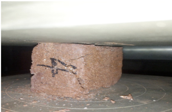
Figure 3. Cracked Block of Clay during Compression Test
