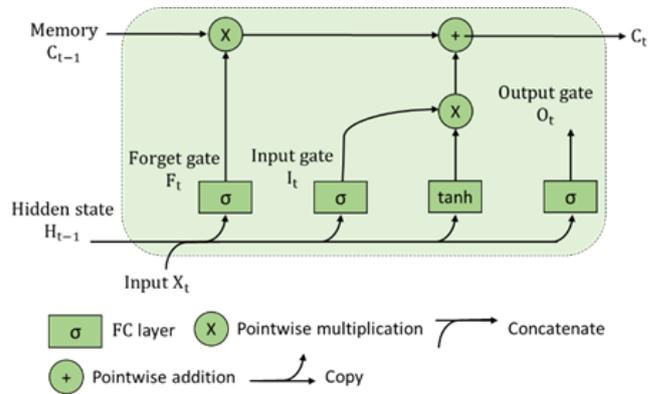
Figure 5. LSTM architecture.
