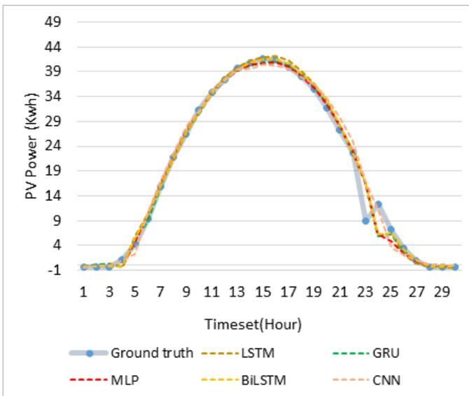
Figure 12. Forecast results on a typical sunny day.
