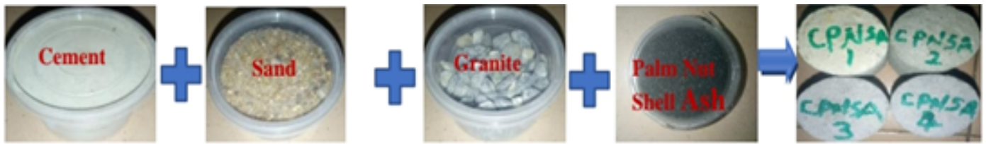
Figure 1. Procedure for the fabrication of concrete samples.
