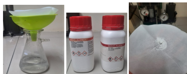
Figure 4: Materials and tools are used in the manufacture of zinc oxide powder by chemical bath deposition (CBD) such as \text{Zn}(\text{NO}_3)_2 and ( \text{C}_6\text{H}_{12}\text{N}_4 ).
